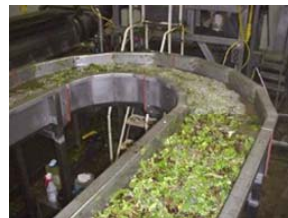
Flume using Ozonated Water
